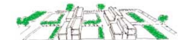
03 - ZEDfactory team propose an additional 1,550m² net workspace on the same 0.64 ha plot. Density is 203 workspaces / ha @ 12m² / workspace, with car pool shared with housing
